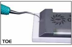
**To shape the toe,** keep the instrument face parallel with the beveled edge then pivot the heel in an arc against the stone.
